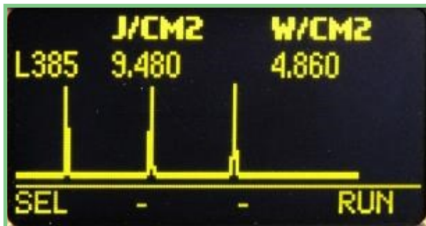
Display showing irradiance & energy density values and the irradiance profile from three LED arrays
